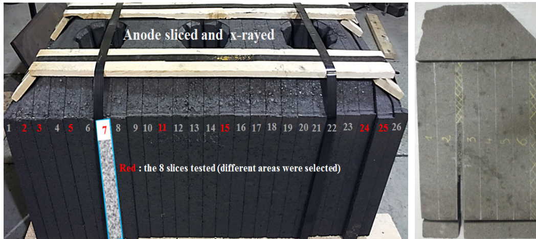
Figure 2. The sliced baked anode. Left: the selected 8 slices are identified in red. Right: example of a slices used for acoustic emission testing.
